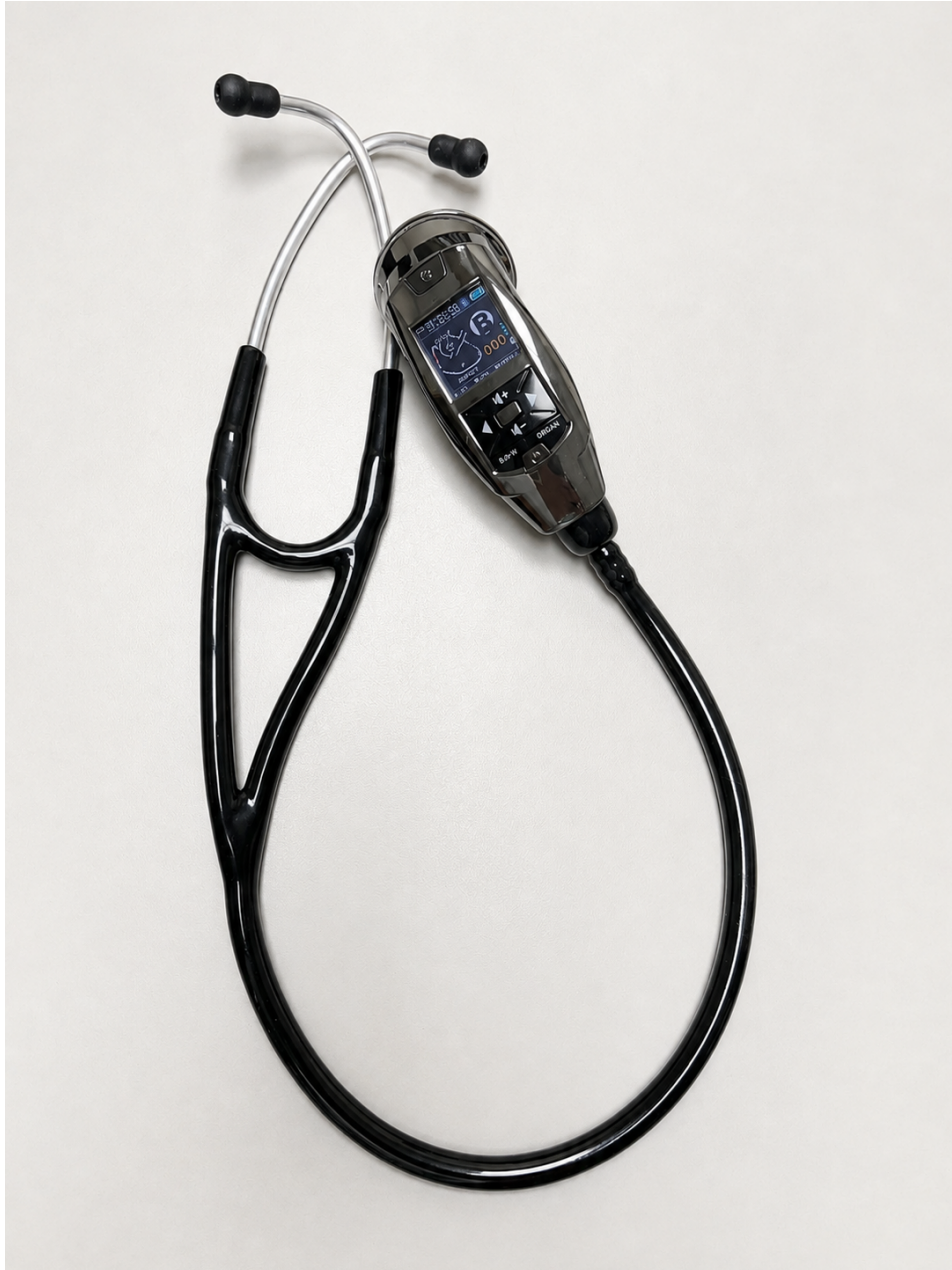
Figure 1. DS101 electronic stethoscope. Photograph of the DS101 electronic stethoscope (Chuang-Xin Medical Electronics) used for arteriovenous fistula acoustic monitoring. The device has a digital display with real-time waveform visualization and connects to a laptop computer via an adapter cable for recording and data transfer.
