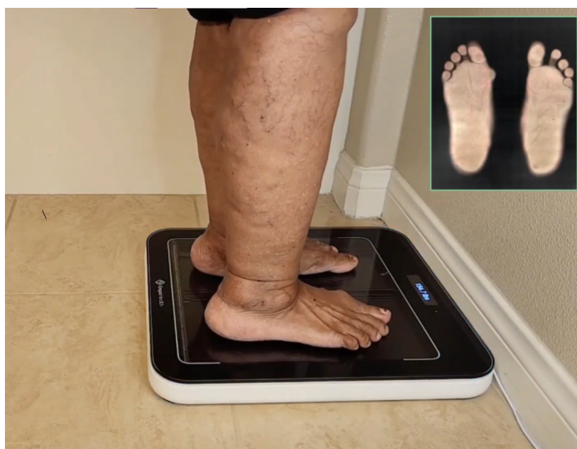
Figure 1. The Empo Footprint with an associated high-resolution, full-color foot scan as uploaded automatically to the Empo Remote Health Link portal.
