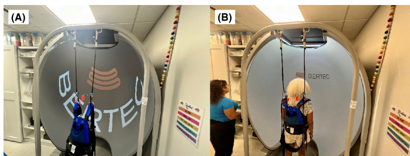
Figure 2. Bertec Balance Advantage system used to conduct monthly sensory organization tests (SOTs) for 2 healthy college students during a 4-month longitudinal feasibility case study (July-December 2023) at the University of Florida. (A) The unoccupied system with the suspended safety harness. (B) A person standing in the system wearing the safety harness for balance assessment.
