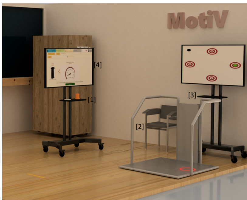
Figure 1. Schematic representation of the measurement and training station of the AS-Tra project featuring a table on which the Polar OH1 pulse measurement device and the K-Force Grip Kinvent hand grip measurement device are placed [1], the aTUG chair [2], the THERA-Trainer Senso training device [3], and the 55-inch touch screen with the app [4]. AS-Tra: Assistance System for sustainable improvement of nutritional and mobility status of older people ( \geq 70 y) under consideration of the transtheoretical model of health behavior change; aTUG: automatic Timed "Up and Go" test.
