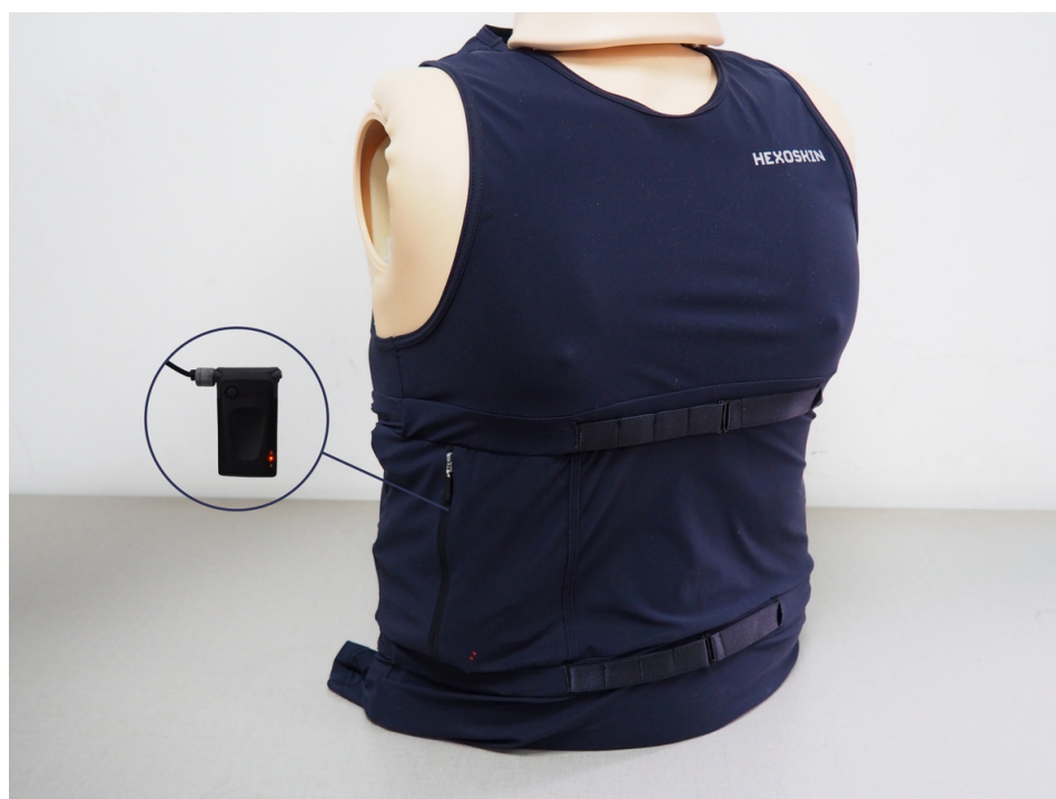
Figure 2. Ambulatory respiratory sensing system. The main image shows the Hexoskin ProShirt embedded with dual-band respiratory inductance plethysmography sensors. The circular inset displays the detachable Hexoskin Smart Device, which functions as the data recording module.
