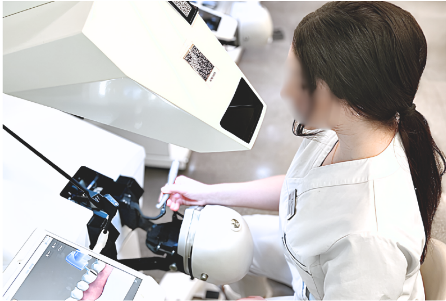
Figure 1. SIMtoCARE Dente screen-based haptic virtual reality simulator used in the study. The system includes a physical handpiece connected to a force-feedback arm and a 3D display-based visual interface.
