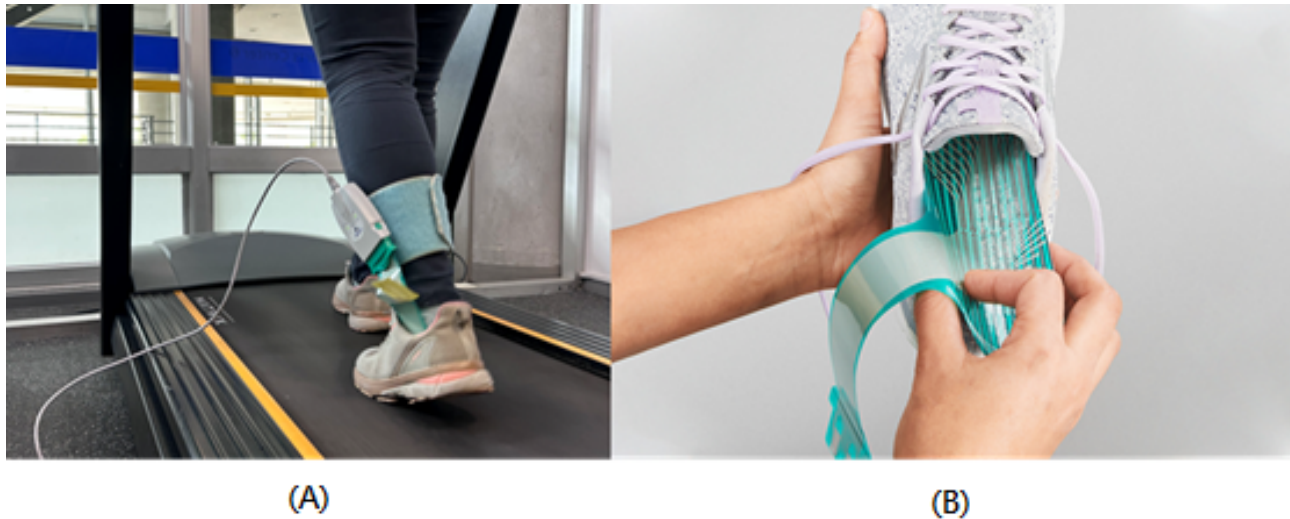
Figure 4. F-Scan plantar pressure sensor: (A) data collection wearing mode and (B) pressure sensing sheet [18].
