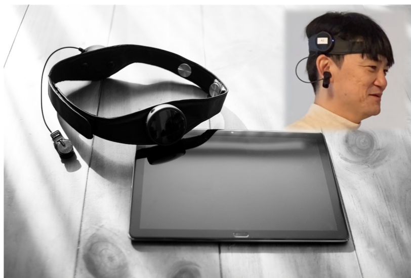
Figure 3. Kansei Analyzer. Left: Kansei analyzer headset and tablet for monitoring emotional status. Top right: example of how the device is worn. The individual depicted provided informed consent for publication of the image.
