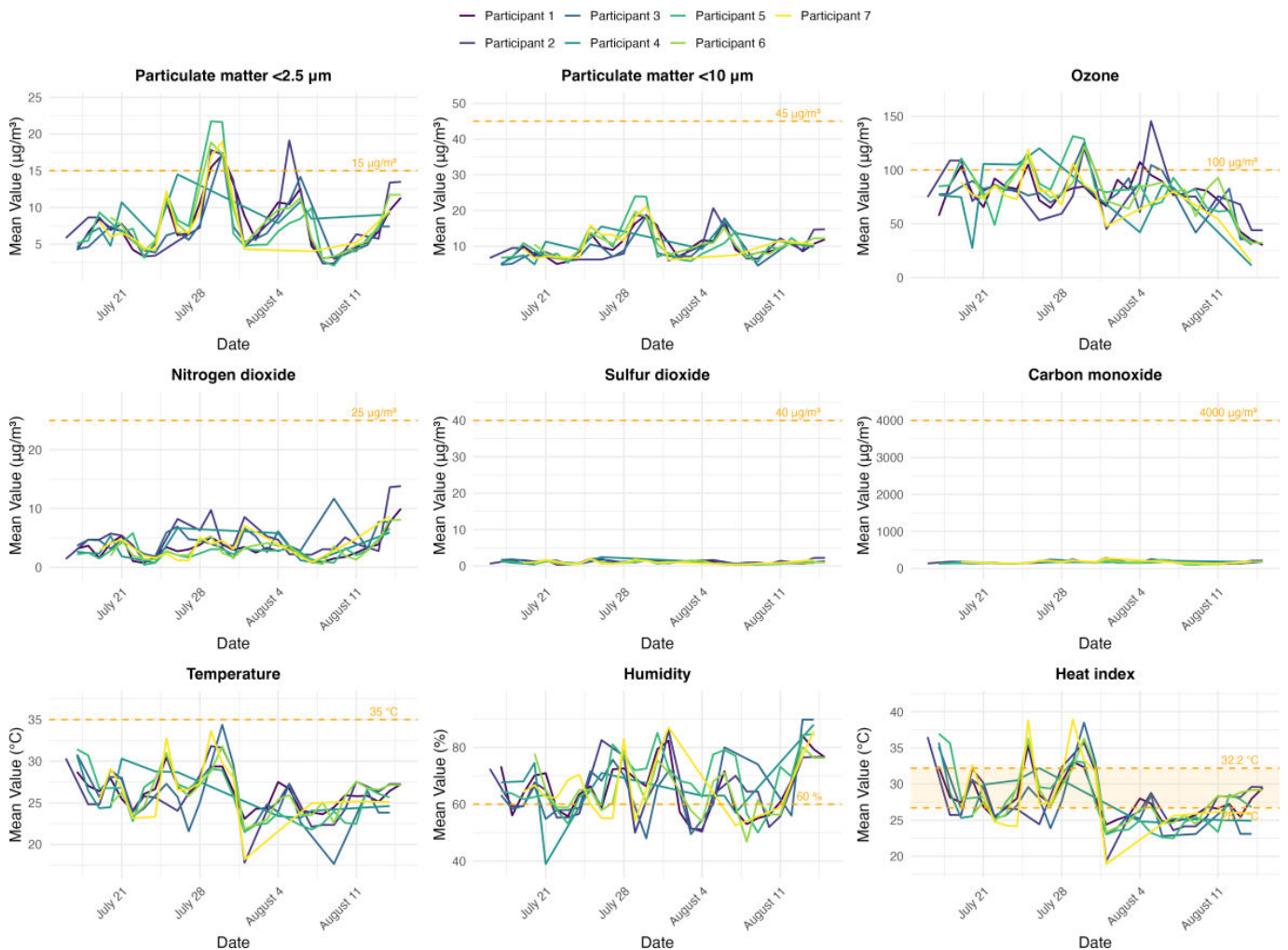
Figure 1. Daily time-weighted average environmental exposures are shown for each participant over the study period, with safe exposure limits indicated by dashed lines. For air pollutants, 24-hour safe exposure limits based on World Health Organization guidelines are shown, except for ozone, for which the 8-hour safe limit is shown. For temperature and humidity, safe limits are shown based on the literature assessing the risk of heat-related morbidity and discomfort. Heat index was derived from Rothfus regression ( ^{\circ}\text{C} ). Aug: August; Jul: July.
