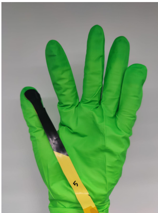
Figure 1. An example of a novel force sensor surgical glove prototype.
