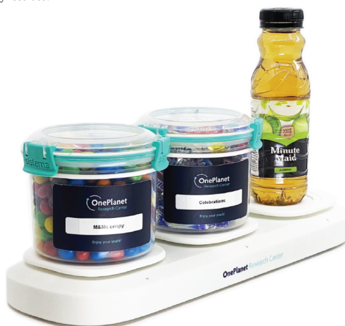
Figure 1. The SnackBox with 3 weighing stations for storing snack containers and beverage bottles. Estimates of consumed quantities and the type of snack or beverage are automatically recorded.
