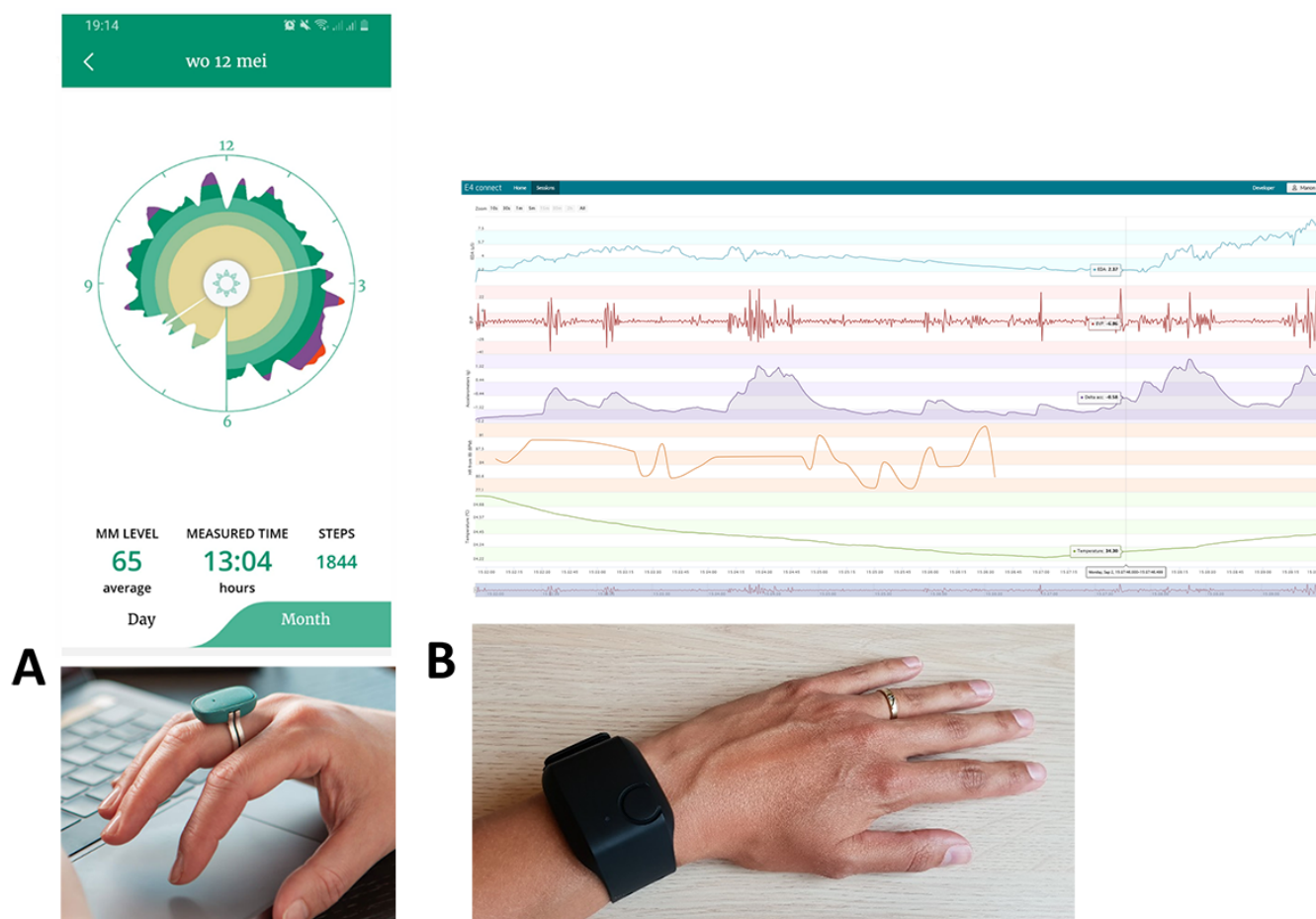
Figure 3. Off-the-shelf technology, which measures stress, was used as a probe to gather the first requirements of end users. (A) The Moodmetric ring with an exemplary visualization and (B) the Empatica E4 with an exemplary visualization.
