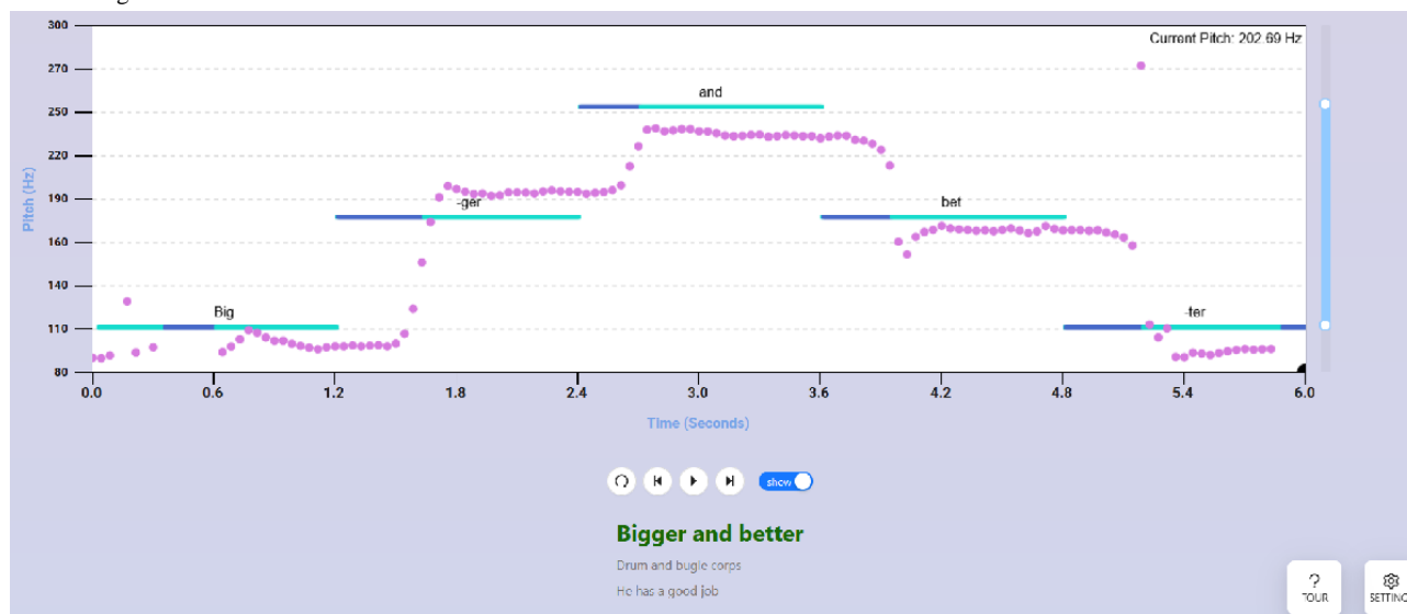
Figure 2. The Stair exercise, which asks the user to match a series of 5 pitch targets. As in the Constant exercise, the user's pitch is by default shown in pink, while the target pitch curve is shown in blue. The target pitch is adjustable with the slider on the right. A show or hide button below the display optionally shows a 5-syllable phrase for the user to speak while matching the 5 pitch targets, and users can move between phrases with next or previous buttons. See Figure 1 for detailed annotation of basic elements.
