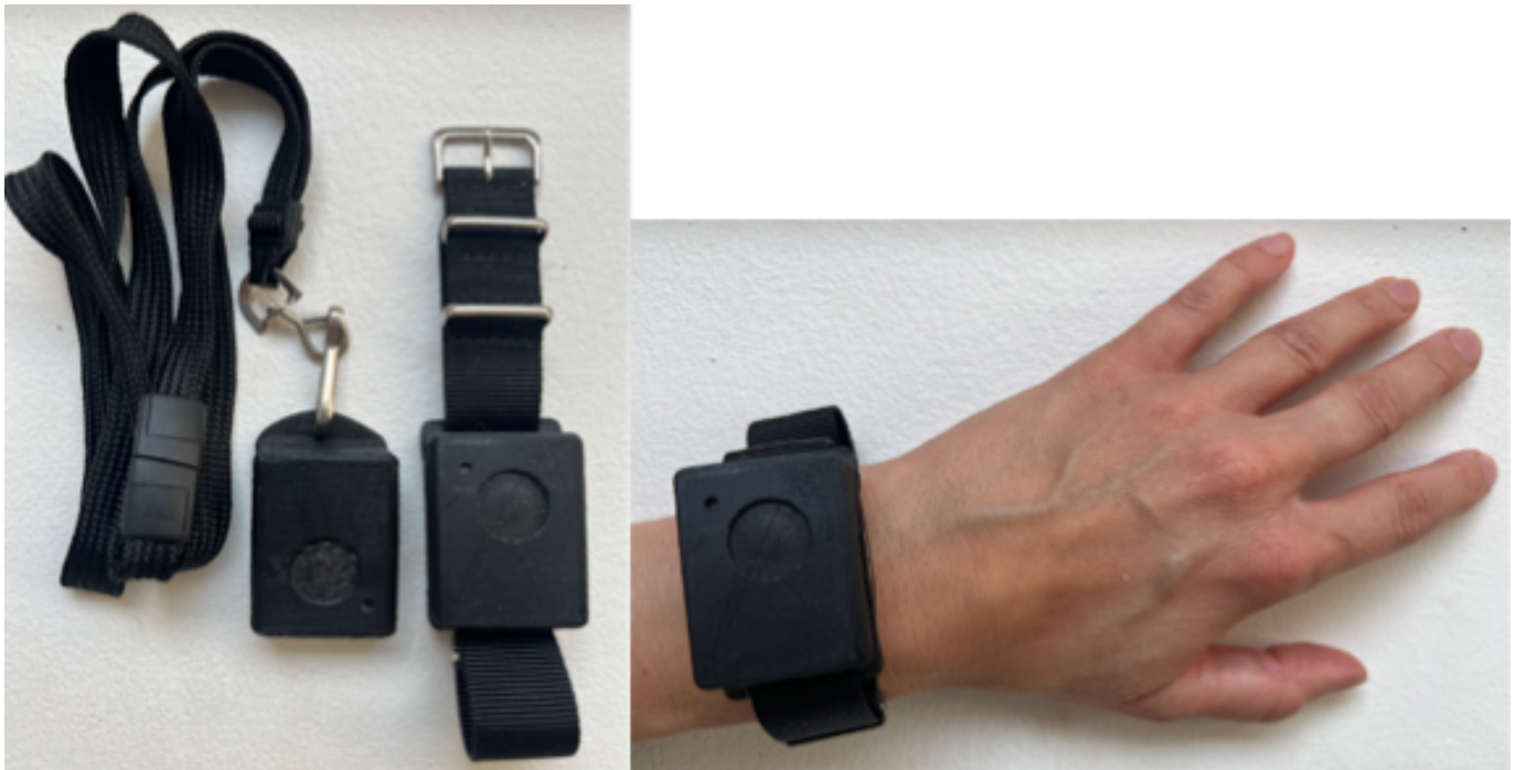
Figure 1. The One Button Tracker, a novel single-purpose wearable self-tracking instrument used in this study, shown configured with a neck strap and wristband.
