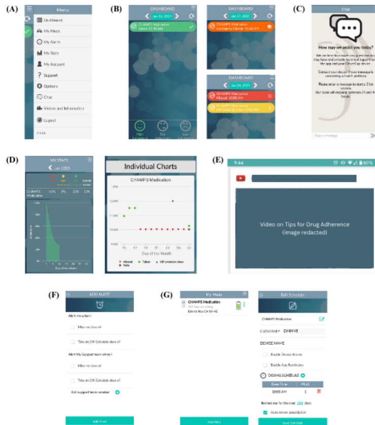
Figure 1. User interface of WiseApp showcasing demo account data: (A) main menu, (B) dashboard with medication adherence status, (C) chat interface, (D) My Stats tab, (E) Videos and Information tab, (F) My Alerts tab, and (G) My Meds tab and Edit Schedule interface.
