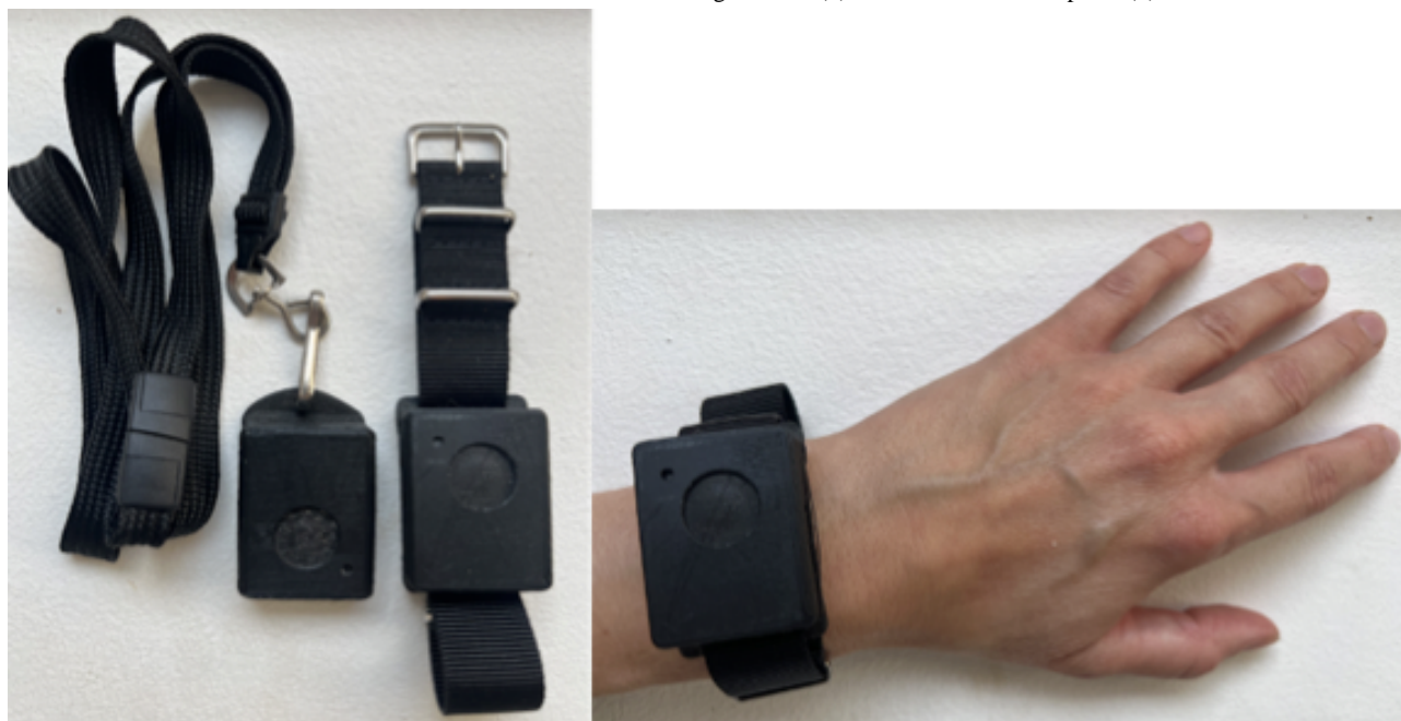
Figure 1. The One Button Tracker instrument shown in two different configurations: (1) worn with a neck strap and (2) worn with a wrist band.
