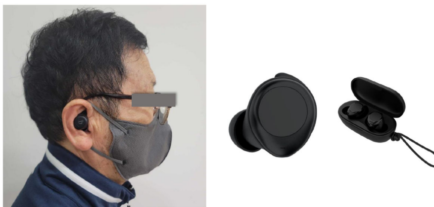
Figure 1. Wearable sensors for gait monitoring (5.7 g, 17.1 \times 20.2 \times 22 \text{ mm}^3 ).
