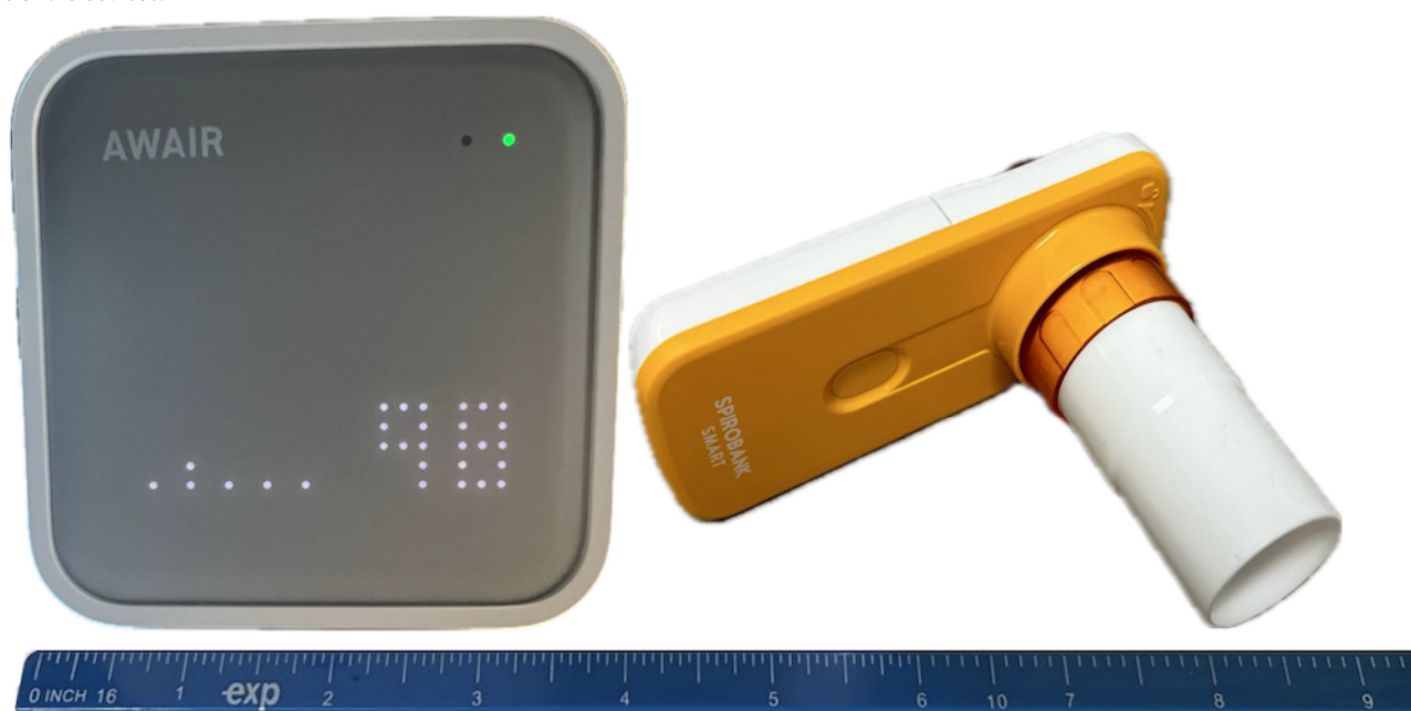
Figure 2. Images of the (A) Awair Omni indoor air quality monitor and (B) the ZephyRx home spirometer. A ruler is included to illustrate the approximate sizes of the devices.
