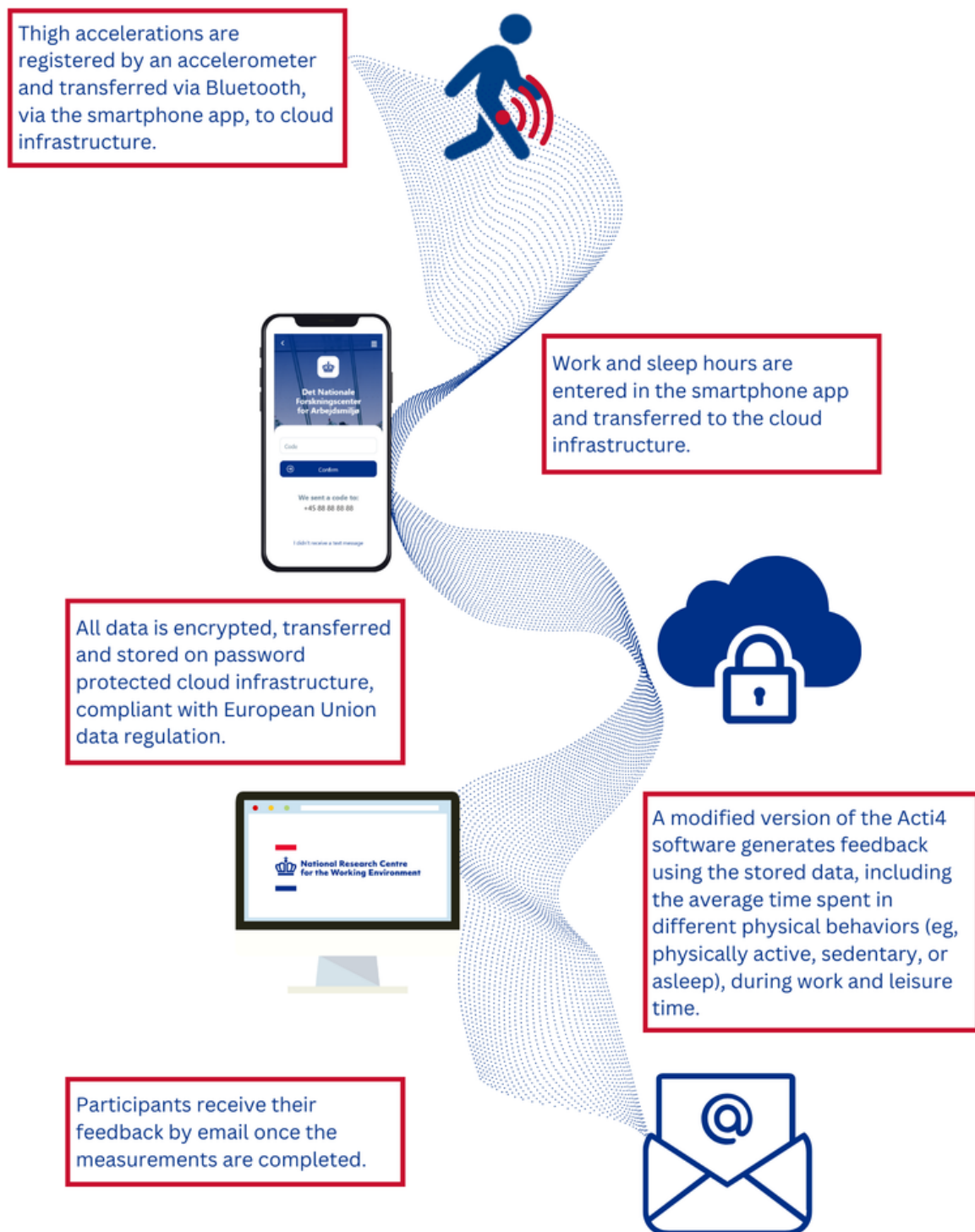
Figure 1. The data flow between the 5 core components of the Motus system. The data flows from the thigh-worn accelerometer, via the smartphone app, to cloud infrastructure.
