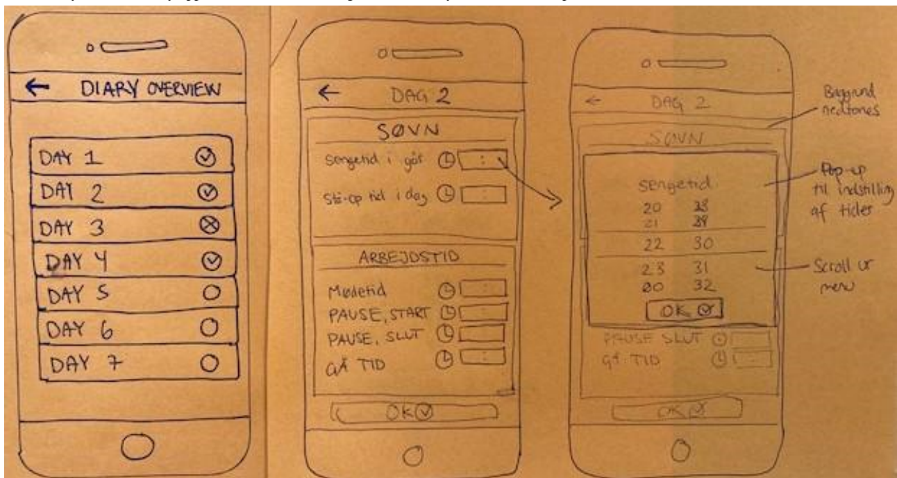
Figure 3. Examples of the initial design ideas illustrated on paper by the project team during the development of the app in phase 1. In this example, ideas for the layout of the diary app screens (from left to right) for the entry of work and sleep hours.
