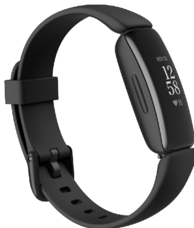
Figure 1. Participants wore a Fitbit Inspire 2 device throughout the study. Sleep data were captured in 1-minute epochs and integrated directly into the WellTap platform engine via an application programming interface. Variables including total sleep time, number of awakenings, wake after sleep onset, sleep efficiency, and sleep timing were included in personalized assessment results presented to patients in the app and to providers in provider reports.
