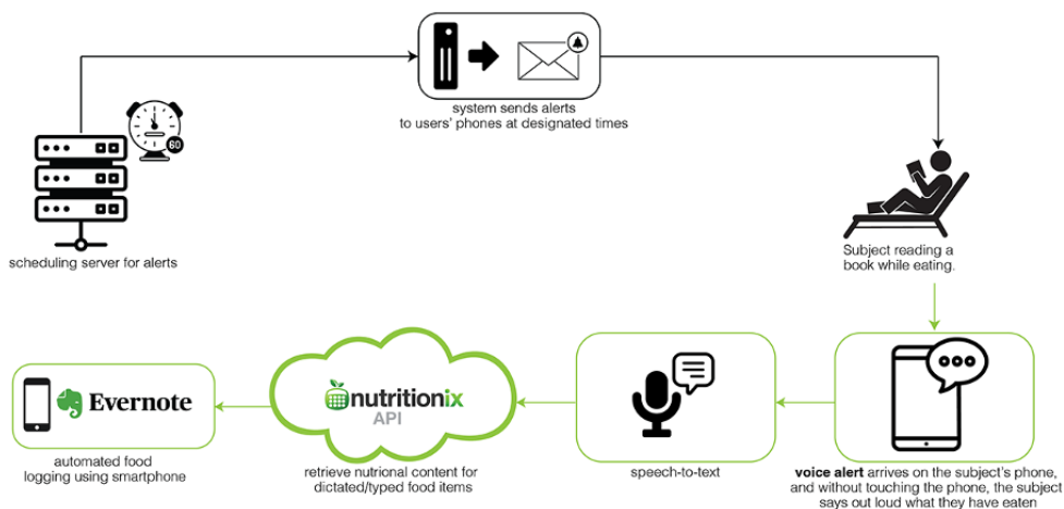
Figure 3. base2Diet app system diagram.
