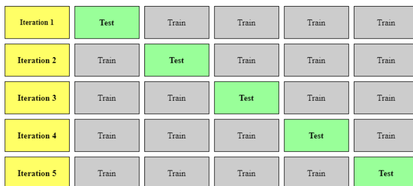
Figure 2. An example of the 5-fold k cross-validation method where k=5. The overall accuracy score is calculated as the mean value of each fold’s accuracy score.
