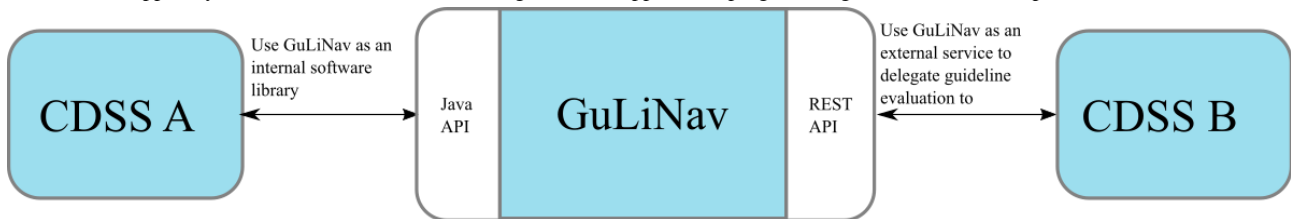
Figure 6. Two distinct interfaces provided by the system: internal software library (Java API) or HTTP (representational state transfer API). CDSS: clinical decision support system; GuLiNav: GuideLine Navigator; API: application programming interface; REST: representational state transfer.
