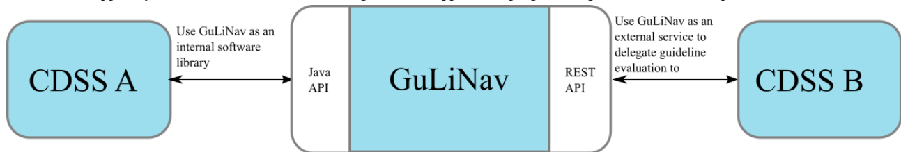
Figure 6. Two distinct interfaces provided by the system: internal software library (Java API) or HTTP (representational state transfer API). CDSS: clinical decision support system; GuLiNav: GuideLine Navigator; API: application programming interface; REST: representational state transfer.
