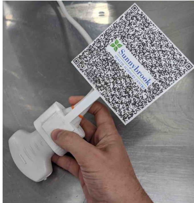
Figure 1. Optical tracking marker attached to a curvilinear probe to enable the HoloLens to detect transducer position.
