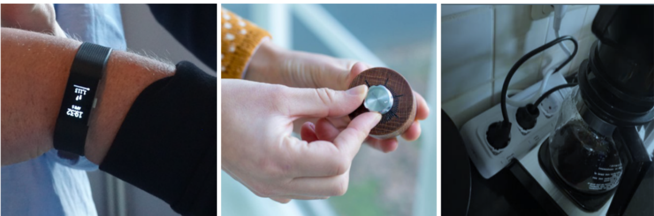
Figure 2. Three examples of trackers used to collect contextual and behavioral data: activity bracelet (left), event button (middle), and smart socket (right).
