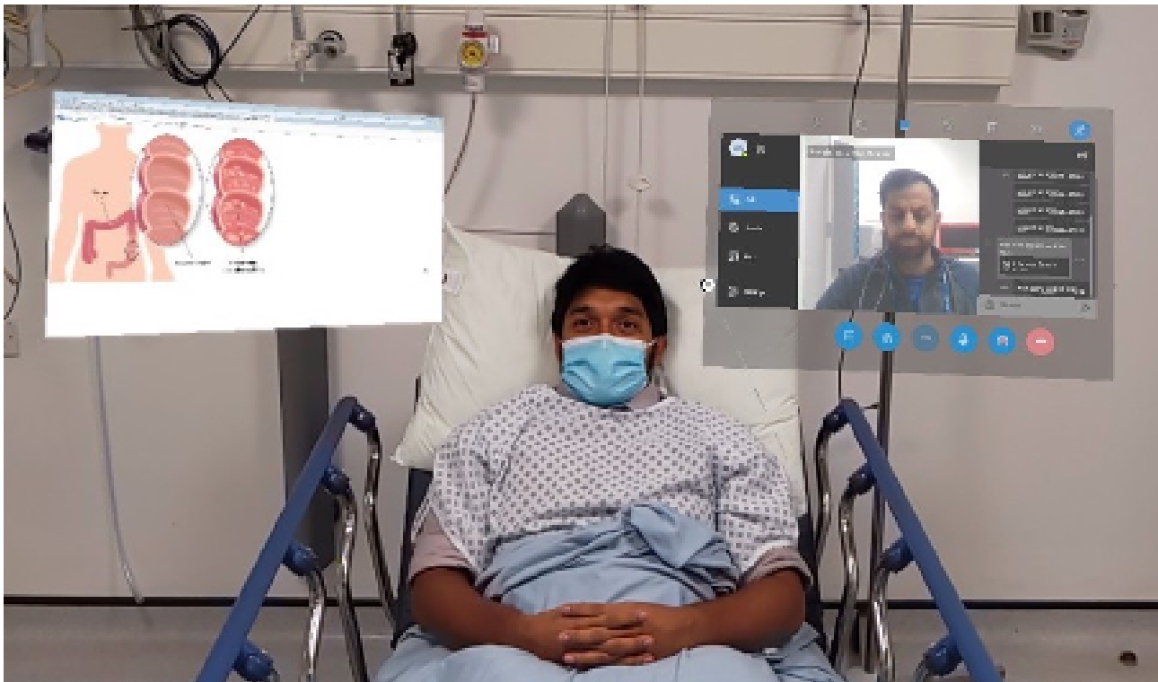
Figure 2. First-person view from the trainer wearing the HoloLens and the same view seen by remote attendee. Video and audio bidirectional communication with trainees occurs through the right screen. Relevant clinical images are shared on the left screen. Both "holograms" can be manipulated by hand gestures (simulated using staff for patient confidentiality, presented with consent by Javed Ahmed and authors AS and AG).
