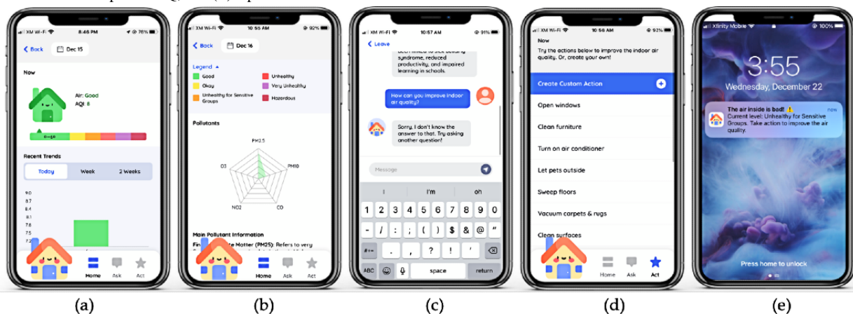
Figure 4. A final design of AirBuddy: (A) a bar graph for indoor air quality (IAQ) history; (B) a spider web for five air pollutants; (C) Airic, a chatbot; (d) a list of actions to improve IAQ; and (E) a push notification.
