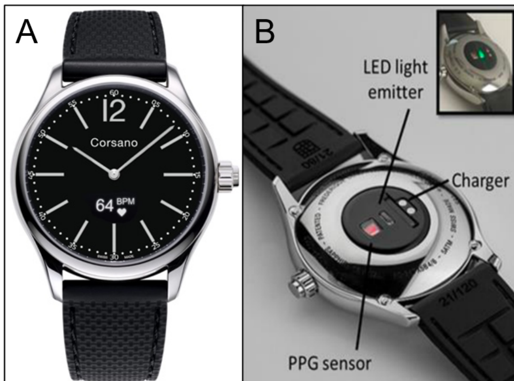
Figure 1. The smartwatch used for measuring photoplethysmographic (PPG) and accelerometric data. (A) A photograph of the front side of the wearable used in the study (Cardio Watch 287, Corsano Health BV). (B) The back side of the device indicating the exact position of the light-emitting diode (LED), the PPG sensor, and the charging contacts.
