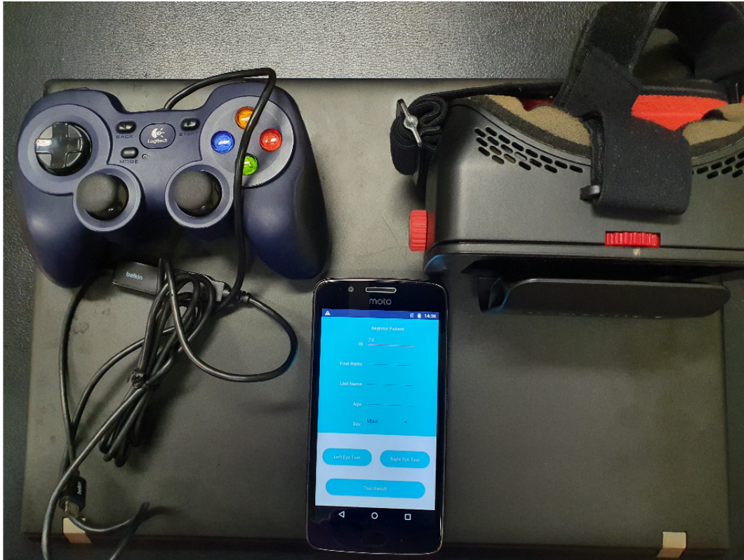
Figure 1. The three components of Glaucoma Easy Screener: smartphone app, virtual reality headset, and joystick.
