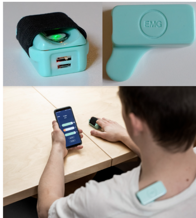
Figure 1. Photos of the wearable sensors. Top left: Combined sensor, measuring peripheral skin temperature and heart rate from the right index finger. Top right: Muscle tension sensor measuring surface electromyographic voltage from the upper trapezius muscle fibers. Bottom: Both sensors in use during a biofeedback session.
