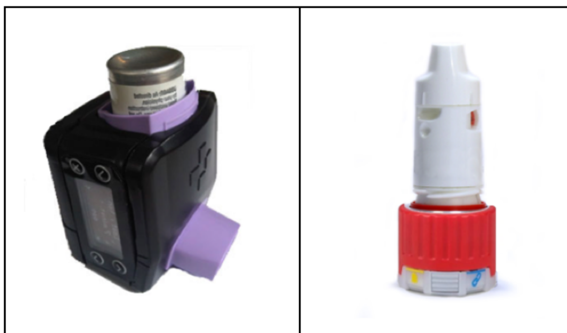
Figure 1. SmartTrack devices connected to pressurized metered-dose inhaler (left) and Turbuhaler inhalation device (right).
