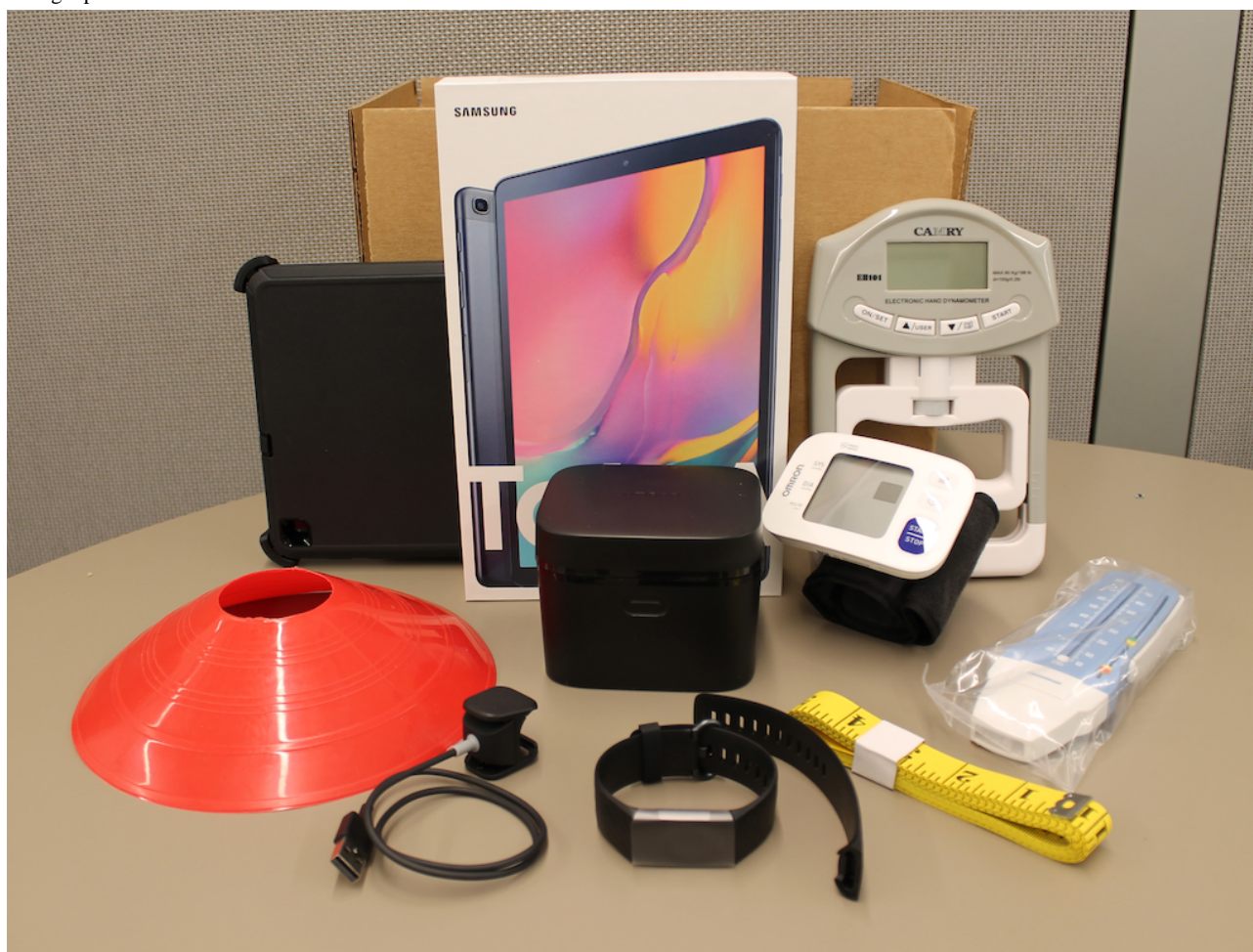
Figure 1. Teleassessment equipment, which included a digital blood pressure cuff, a hand dynamometer, a spirometer, a mini disc cone, and a 3-meter measuring tape.
