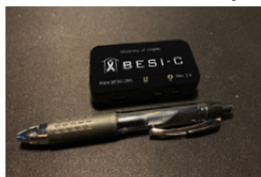
Figure 3. Behavioral and Environmental Sensing and Intervention for Cancer (BESI-C) updated environmental sensor based on user design input. The image shows a smaller, black, rectangular device with the BESI-C logo and text on its surface, placed on a dark surface next to a pen for scale.
