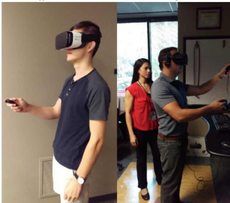
Figure 1. Samsung Oculus Gear VR with supplemental hand controller (left) and Oculus Rift (right).
